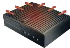
Aluminum housing for superior heat dissipation
