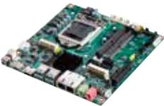
Intel® Core™ i7/i5/i3 LGA 1151 Mini-ITX, 2 COM, 双LAN, PCIe x4, miniPCIe, DDR4, DC Input
